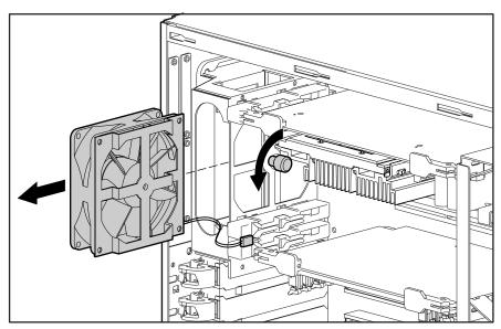
Figure 2-14. Removing the rear fan
